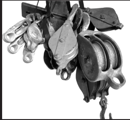
Block and tackle & heavy steel pulleys
